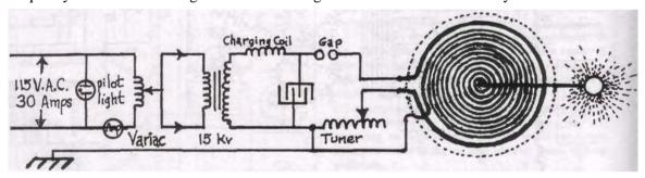
This 150 kv coil design has a single-turn primary and 10-turn secondary (1:10 ratio), with a maximum voltage increase of 15 kv per turn of the secondary. 1/8" increased spacing per turn is sufficient, using a dielectric with a K-value of 4. The secondary wire will be about 1/8" in diameter, and the primary will be a 1/2" wide copper strip about 1/32" thick. The following schedule of spacing between turns is observed:
