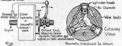
Not shown in the request for amendment or drawings, the two different valve plungers---17 of FIG 1, and 68 of FIG 4---should be replaced with the same 'push-pull'-type tapered plungers and seats, on both embodiments 1 and 1a, as follows:
