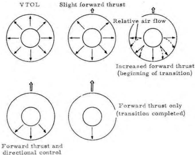
Fig 5. Changes of airflow during VTOL and Transitional flight.
