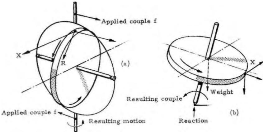
Fig 51. The dynamics of a spinning top.
