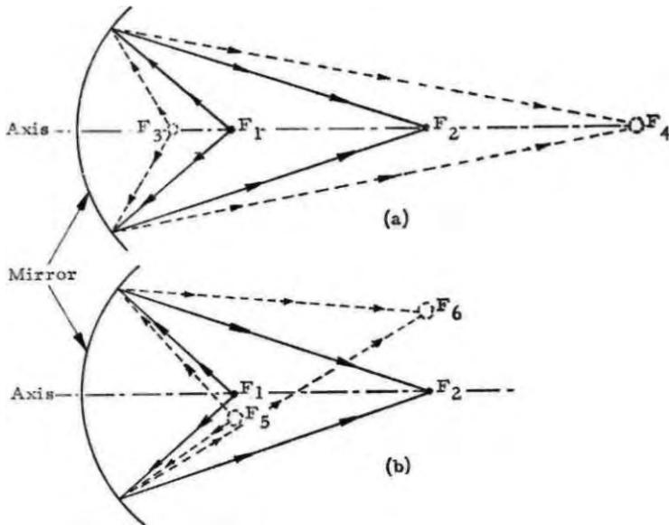
Fig 54. The fundamentals of optically focusing a beam of light to a variable focal length.
