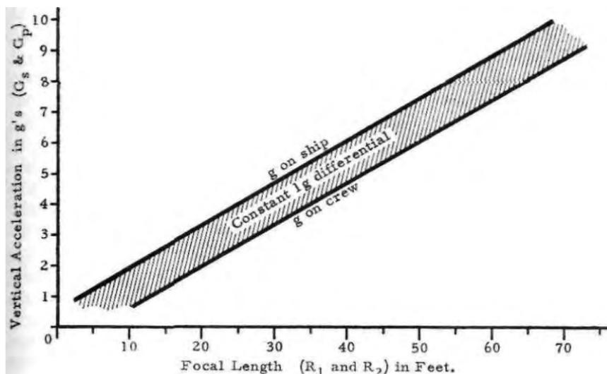
Fig 74. Varying focal lengths for a constant ship-crew differential of  $1g$ .
