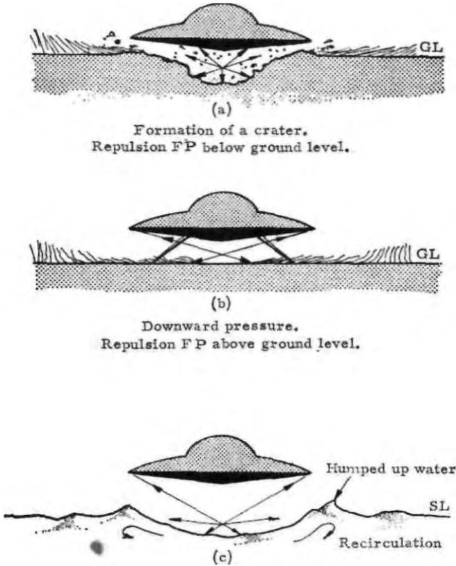
Fig 67. Surface effects due to a repulsion point source.
