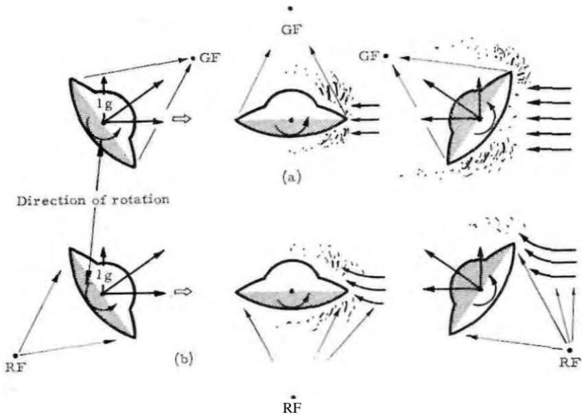
Fig 92. Rotating the machine would reverse the field thrust, but would not obviate aerodynamic forces.
