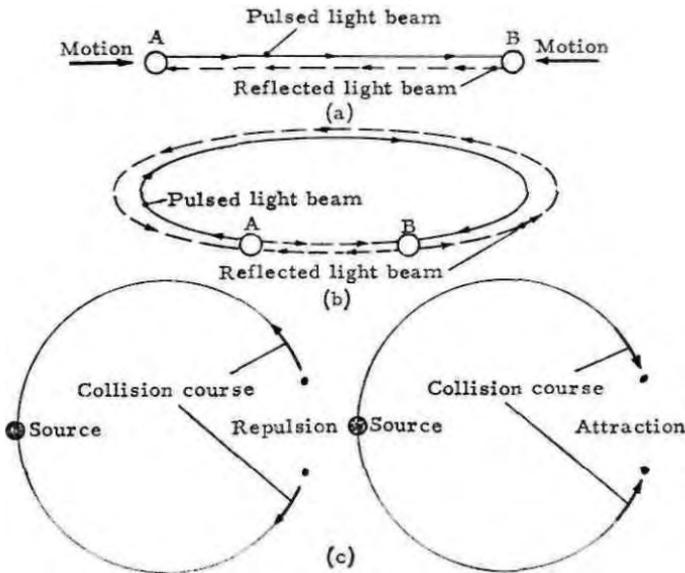
Fig 18. Whatever their relative motions may be, two moving bodies are on a collision course when considered from the source.
