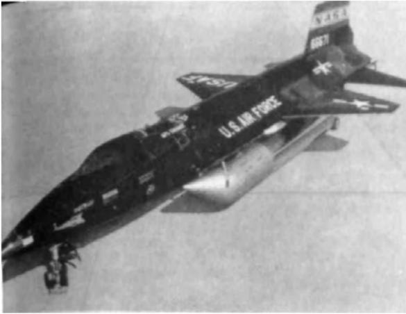
Plate 1. Rocket powered North American X-15 high altitude hypersonic research aircraft.
