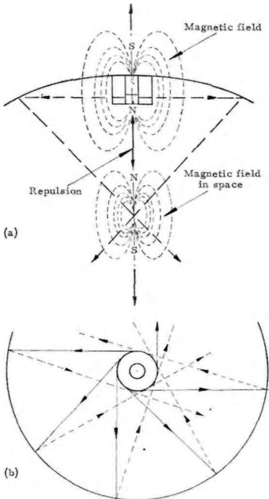
Fig 62. Analogous repulsion of an isolated magnetic field.
