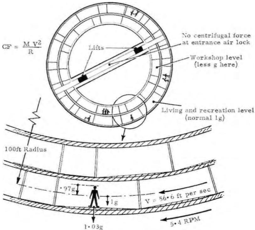
Fig 33. Differential centrifugal stress on the body in a rotating space station.
