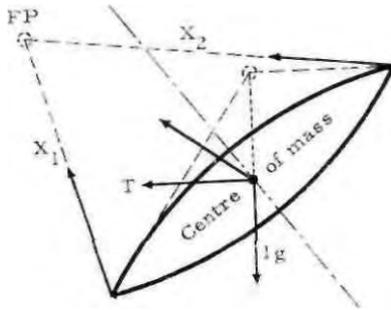
Fig 55. Asymmetrical forces about the centre of mass, due to displaced focal point.
